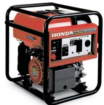
Honda 6.5-hp, 3,000-watt commercial generator features full GFCI circuit protection, CycloConverter technology which makes it dramatically lighter than other units producing the same amount of power weighing 68.4 lbs., fuel gauge, DC charging, and oil alert. 18 29 / 32 "H x 15 3 / 4 "W x 17 7 / 16 "L Item 752464
